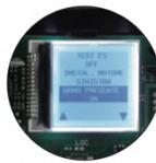
SELF-PROGRAMMING MONITORED BY AN LCD GRAPHICS DISPLAY
